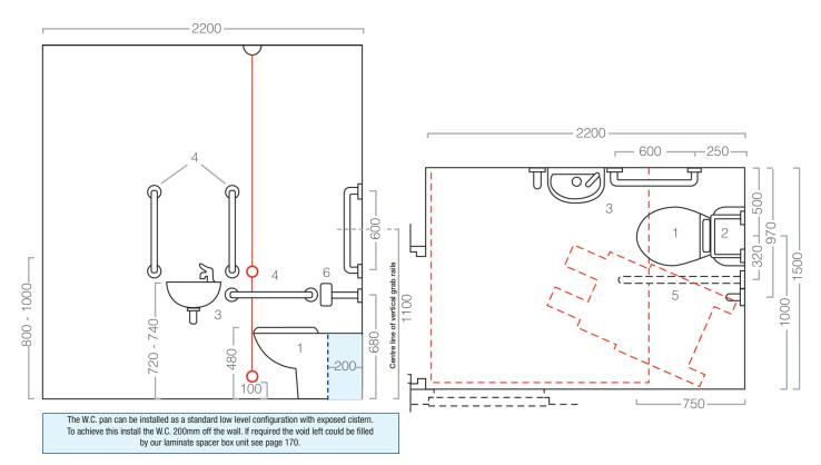
Cistern lever should be installed on the right of the cistern for LH installation and on the left for a RH installation. (Left hand illustrated.)
