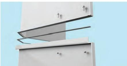
Place gasket between the shower wall sections and tighten bolts.
