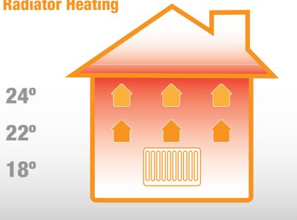
Standard heating systems within homes such as radiators work by heating the air surrounding them using convection. The air is heated by the radiators, travels up to the ceiling and cools and falls back down to ground level to start the cycle again. However, this system allows specific areas nearer to the radiator to become overheated which of course is inefficient and expensive.
