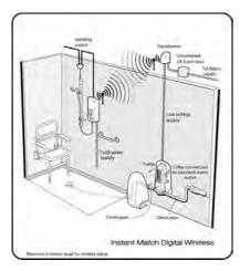
To minimise gulley suction noise the Whale Instant Match uses a digital signal sent from the Mira Advance Extra to automatically adjust the pump speed in relation to the flow rate of the shower.
