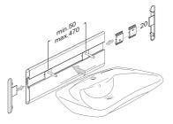
Mounting of wash basin: Bolt-mounted basin. Basin hole spacing: Min. 50mm; max. 470mm.
