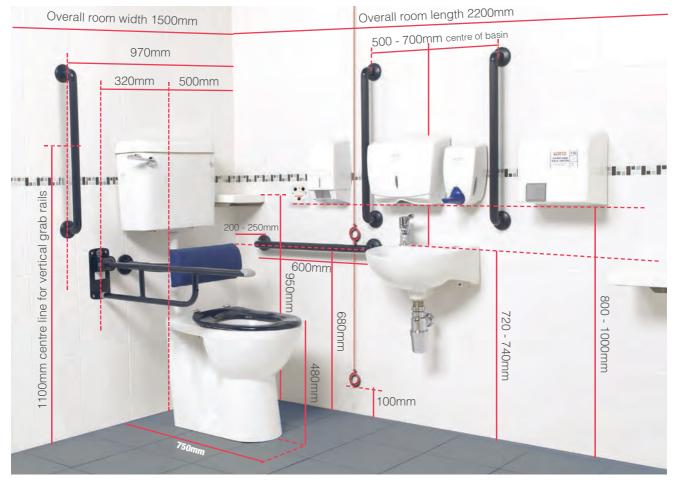
Consideration should also be made for the positioning of equipment for both wheelchair and ambulant users. The BS8300 is very prescriptive in these measurements and requirements. N&C Phlexicare provides these dimensions in technical drawings contained within each MPack box supplied.
