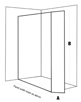
To achieve a corner wall screen with a mobile panel, please order the size of panel from above and add a mobile panel (6mm glass).
