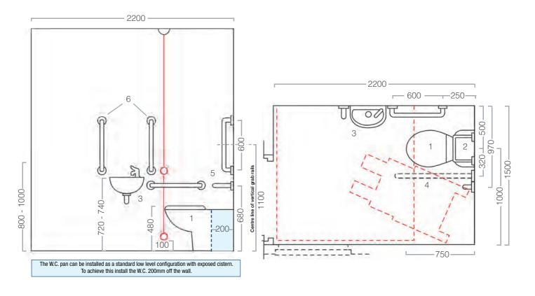
Cistern lever should be installed on the right of the cistern for LH installation and on the left for a RH installation. (Left hand illustrated.)
