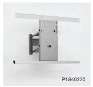
Electric lift for wall cupboards 400 to 1200mm wide. The diagonal adjustment has a single motor with two cross braces allowing a cabinet to move down by 430mm and forward by 180mm.
