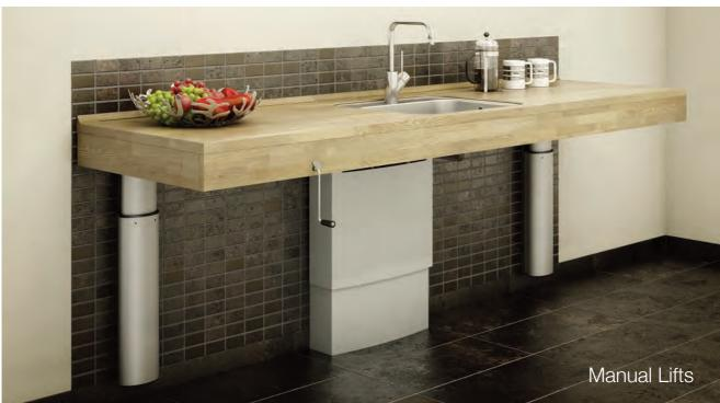
Our Indivo manual wall mounted frames are available in any length up to 3000mm. It is advised, but not essential, that a 100mm high worktop plinth be fitted beneath the worktops front and return edges to accommodate a manual crank. If a worktop plinth is not required, a collapsible crank handle must be ordered. Total loading capacity including worktop is 100kg. Height adjustment ranges from 630mm to 930mm.
