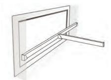
The simple addition of our Window Spanning Kit allows a wall fixing for a shower curtain track, or a wall bracket from one of our Pro-door options, to be fixed where a window would otherwise obstruct thier installation. Our Window Spanning Kit also doubles up as a curtain track, with hooks and gliders.
