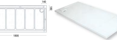
The 1800mm Quick Fit Shower tray can be cut down to a minimum of 1500mm as there are metal strengthening bars that cross the tray at 100mm intervals and comes complete with end panel section. This allows greater flexibility for onsite conditions and allows one tray to be provided for many different scenarios, e.g a 1560mm alcove can be catered for by cutting an 1800mm tray to the exact size required and then fixing the finished end panel section. .
