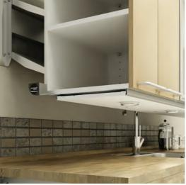
A pressure sensitive safety plate installed beneath the wall cabinets will suspend downward movement if resistance is encountered. The unit will then automatically rise by 10 to 30mm releasing tension between the safety stop and obstruction.
