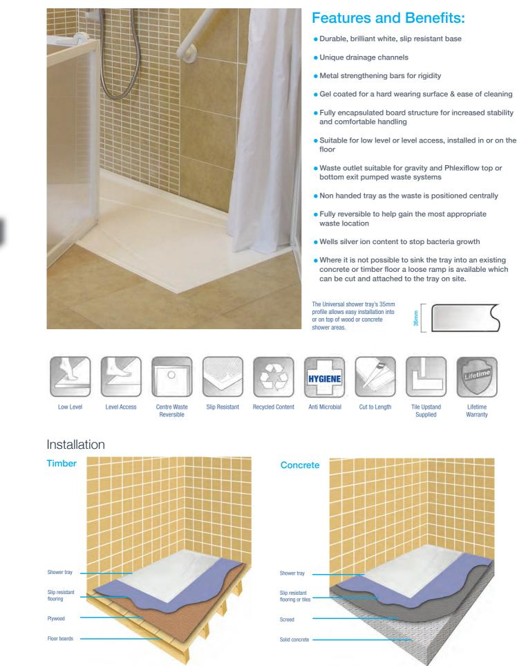
The Universal Shower Tray can be sited directly onto the timber floor for low level access or alternatively the boarding can be removed and the tray sunk into the floor. With a combination of plywood and the preferred finished flooring, level access can be achieved. The Universal Shower Tray can be sited directly onto the screed for low level access or alternatively the screed can be removed and the tray sunk into the floor for level access.
