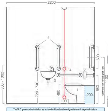
The W.C. pan can be installed as a standard low level configuration with exposed cistern. To achieve this install the W.C. 200mm off the wall. If required the void left could be filled by our laminate spacer box unit see page 170.
