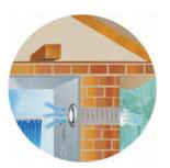
The rate of extraction you require depends on the size of the room and the amount of condensation produced. The bigger the room or if large amounts of condensation are produced, then the more the air will need to be replaced in the room, thus you need a higher rate of extraction.
