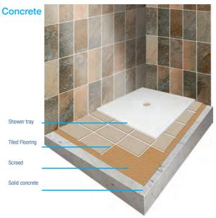
The Trimline shower tray can be installed into an existing timber floor by removing the floorboards and setting the tray onto the joists and in-fill panels. The tray will then be brought level with the existing floor with Plastic Ply/plywood to make the whole shower room level. May also be placed directly on top of the existing floor. Low level access can be achieved if installing onto existing concrete floors. Trimline tray can be sited directly onto the concrete or screed subfloor.
