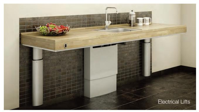
The Indivo electric wall mounted frames are available in any length up to 3000mm. It is advisable, but not essential, that a 100mm high worktop plinth is fitted beneath to accommodate the electric switch and safety stop. Total loading capacity including worktop is 100kg. Height adjustment ranges from 620mm to 900mm. All electric models come with safety stop as standard. Electric 'L' shaped frames are also available.
