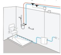
The Phlexiflow High capacity pump is the ideal solution for power showers with an output between 12 - 20 litres per minute.
