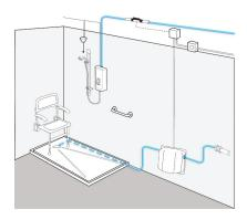
This standard kit comes with a flow switch. Factory pre-set to allow 7-9 litres of water per minute to be removed. It can be adjusted on site to cope with up to 12 litres per minute. For a mixer valve, 2 flow switches are required.
