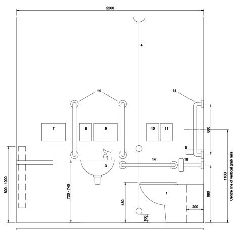
The W.C. pan can be installed as a standard low level configuration with exposed cistern. To achieve this install the W.C. 200mm off the wall. If required the void left could be filled by our laminate spacer box unit.
