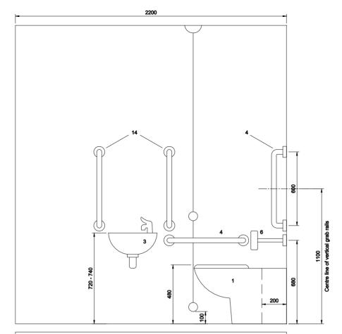
The W.C. pan can be installed as a standard low level configuration with exposed cistern. To achieve this install the W.C. 200mm off the wall. If required the void left could be filled by our laminate spacer box unit.
